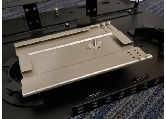
Figure 10: ST-01 splice tray(sold separately) installed. Note the winged nut must be screwed on after the splice tray cover. But can be used as shown without cover for holding in place while splicing.
