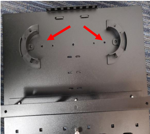
Figure 8: Multiple positions allowed for screwing in cable management spools around splice tray
