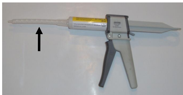
Figure 5d Static Mixer Installed on Dual Cartridge
