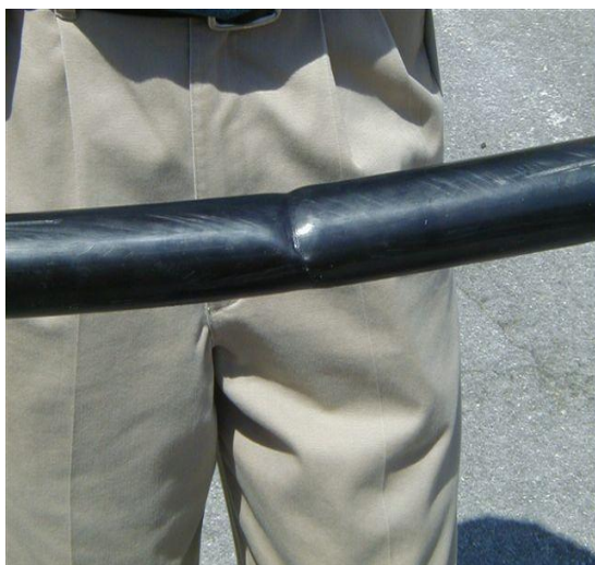
Figure 1 Badly Kinked Tube Cable
