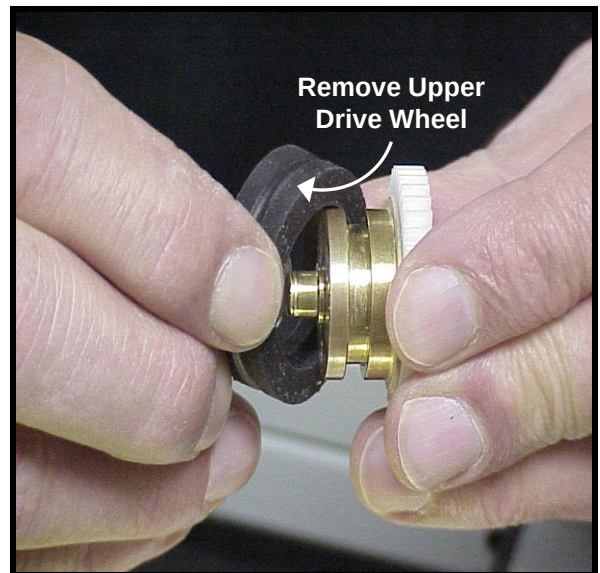
Figure 43 Remove Upper Drive Wheel from Hub
