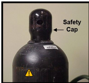
Figure 8 - Safety Cap Installed
