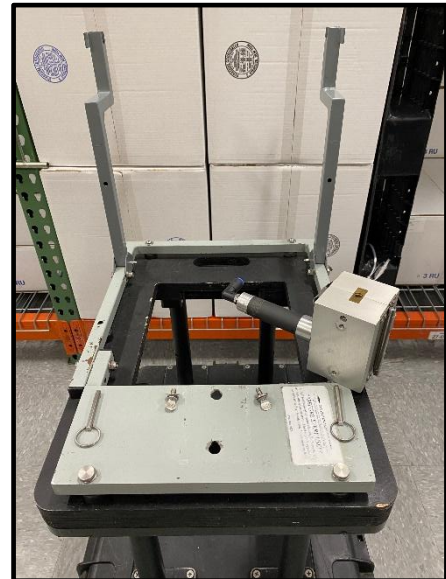
Figure 53 Blowing Head Shown Removed from the Payoff Stand Shelf
