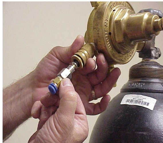
Figure 3 8mm Tubing Adapter Installed to Pressure Regulator
