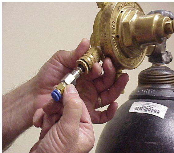
Figure 3 8mm Tubing Adapter Installed to Pressure Regulator
