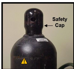
Figure 8 - Safety Cap Installed
