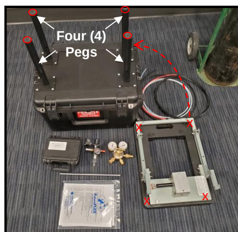
Figure 6 All BH Kit contents removed from the case. Pegs/Supports installed on the top of the Transit Case lid into predesignated holes.
