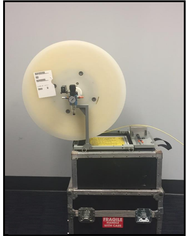
Figure 58 Properly Mounted 72-Fiber Reel on an Assembled Transit Case
