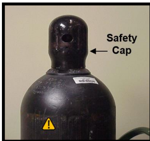
Figure 8 - Safety Cap Installed
