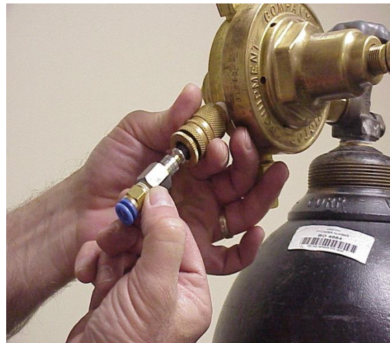
Figure 3 8mm Tubing Adapter Installed to Pressure Regulator
