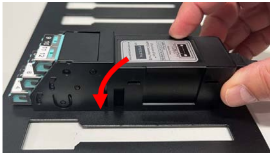
5.1 Hold both the left and right latch (black color) and pull the slide chassis to the front.
