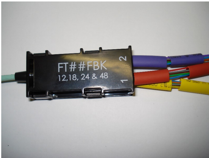
Figure 6 Fiber Bundle Foam & Nylon Jackets Even With or Just Forward of 3 mm bushing
