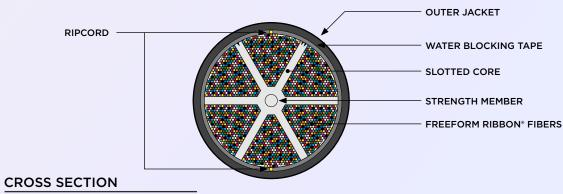
Freeform Ribbon® Conventional OSP All-Dielectric Slotted Core Cables
