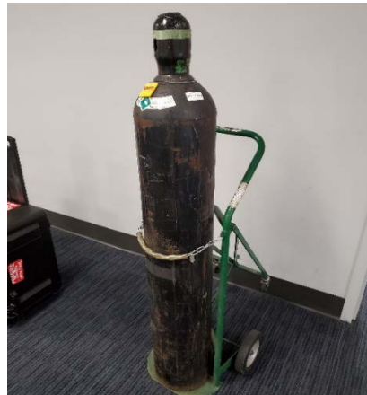
Figure 1 Strapped and Capped Nitrogen Tank
