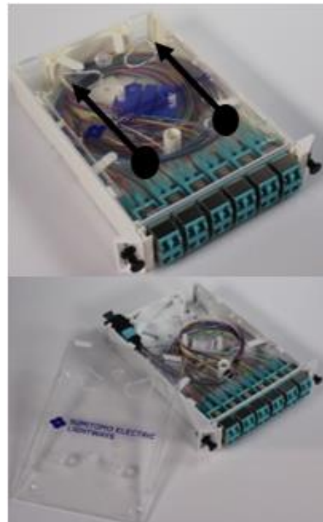
Figure 4 Firmly press thumbs down where black dots are on clear lid and slide lid towards back of cassette (away from faceplate).
