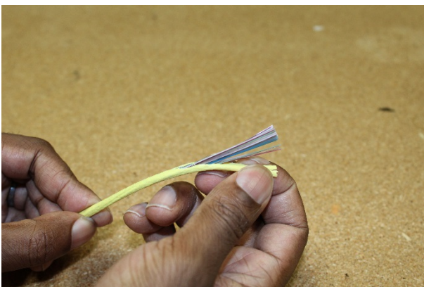
Figure 2 Breaking into a Fiber Jacket by Hand
