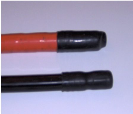
Figure 2 Heat Shrink End Caps Installed
