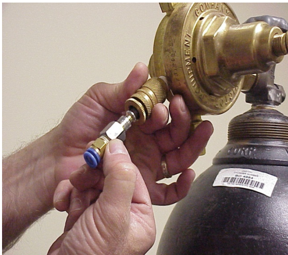
Figure 3 8mm Tubing Adapter Installed to Pressure Regulator
