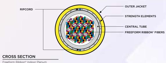
Freeform Ribbon® Indoor Plenum Central Tube Cables
