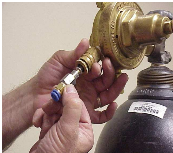
Figure 3 8mm Tubing Adapter Installed to Pressure Regulator
