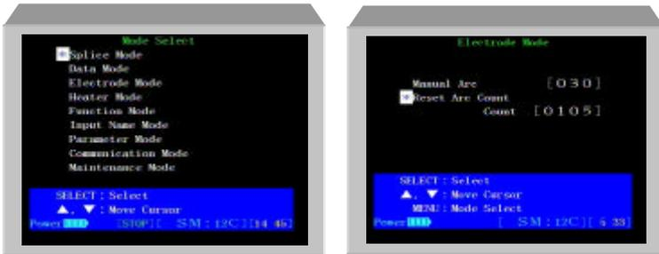
**Figure 33. Displaying Electrode Mode Screen**
