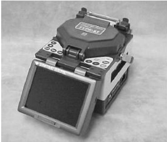
**Figure 1. Type 65 Fusion Splicer**
