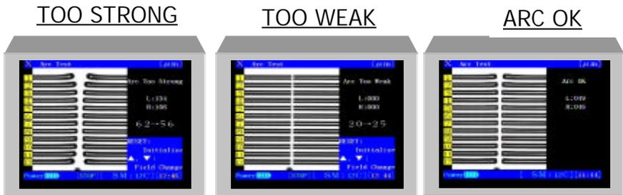
Figure 21B. Performing an ARC Test
