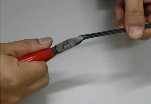
1. Separate the steel wire from the cable using nippers.
