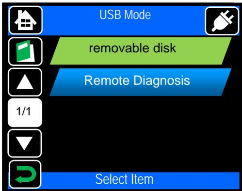
Touch USB icon (
