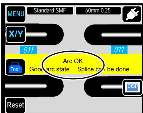
8: If “Arc OK” is displayed, begin the fiber preparation procedure to perform a splice. The splicer automatically initializes when the hood is opened.
