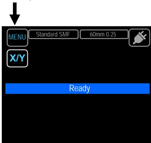
Remove the spliced fiber when the screen above is displayed.
