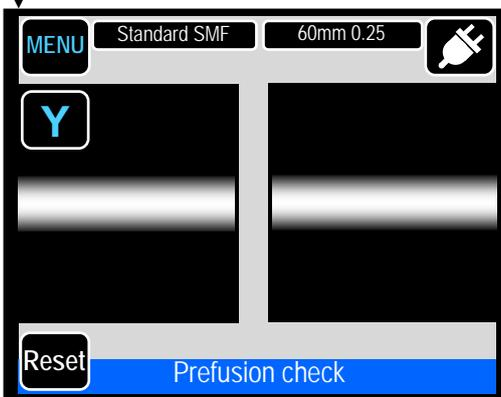
Inspection of fiber end face & dust
