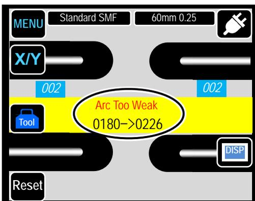
7: If “Arc Too Weak”, “Arc Too Strong” or “Arc Center” is displayed, prepare the fiber again and repeat the test until “ARC OK” is displayed.
