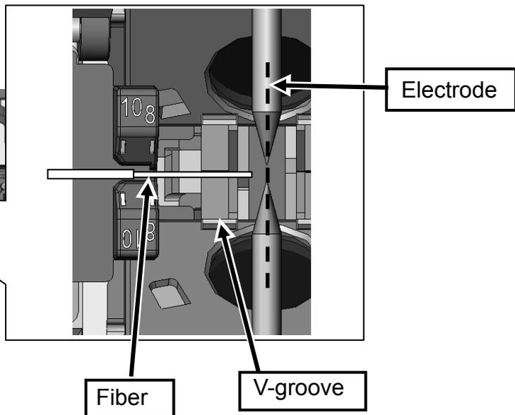
1: Set the fiber end between the edge of v-groove and the electrode.
