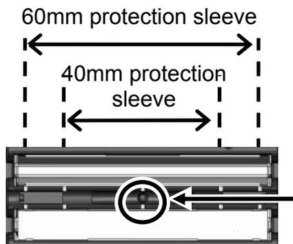
Marking for the center of the heat shrink oven
