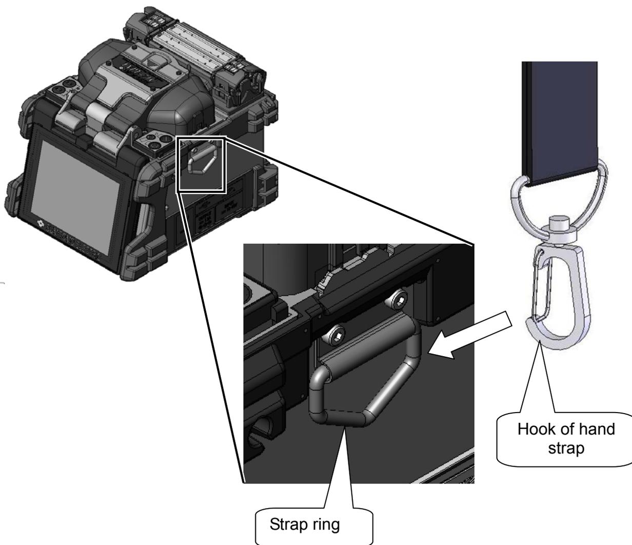
Please pass the hook at both ends of the hand strap through a right and left strap ring of TYPE-Q101-CA.
