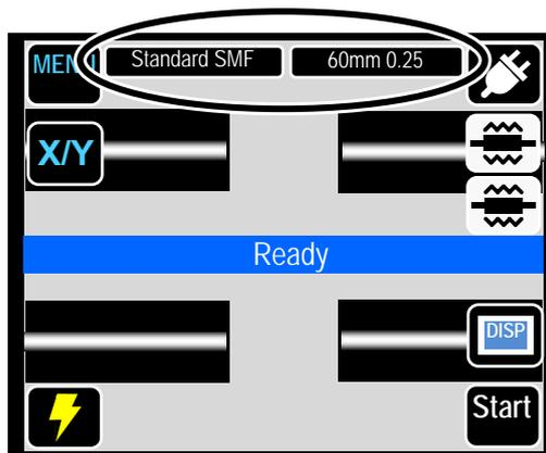
1: Set each fiber that has been prepared. (The coating is removed and fiber is cleaved.)
