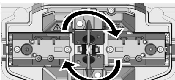
2. After replacing right and left holder stage, tighten the holder stage fixation screw. The lid of the fiber holder opens in the same direction as the front monitor type from the operator's position.
