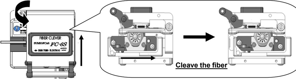
Lower the top clamp lever. Slide the blade carriage to the rear of the cleaver as indicated by the arrow.
