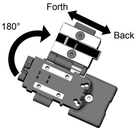
2. The lid can be moved back and forth by opening the coating clamp lid by 180°. Change the position of the lid according to the coating of the fiber, and the shut the lid.
