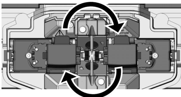
2. After replacing right and left coating clamp, tighten the coating clamp fixation screw. The lid of the coating clamp opens in the same direction as the front monitor type from the operator's position.
