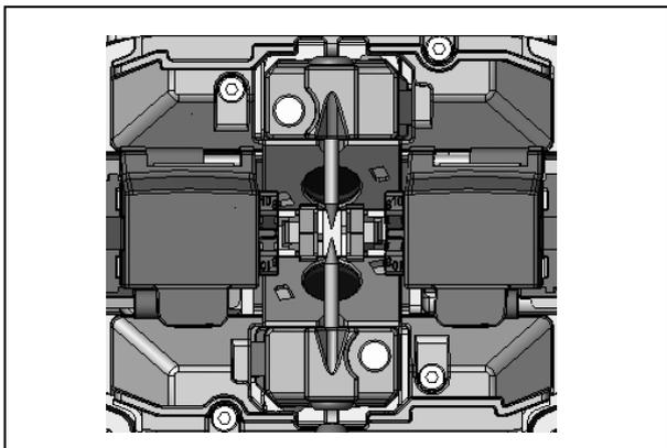
6: Tighten the thumbscrew while pressing the electrode below at each electrode cover plate.
