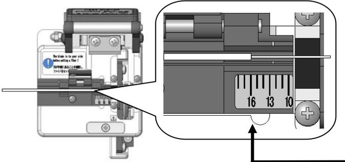
Lower the fiber into the correct V-groove with the end of the fiber coating (e.g. if the cleave length is 16mm) **at the 16mm mark on the ruler.**
