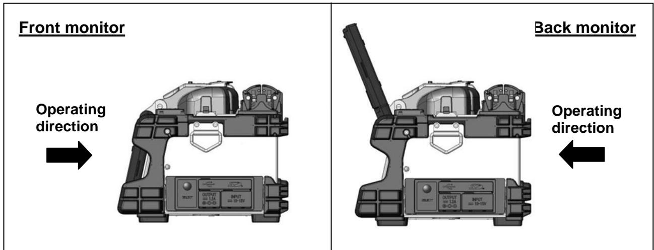
The monitor display reverses automatically when the monitor is moved to the position of the back monitor type. (Refer to the page 4-10)
