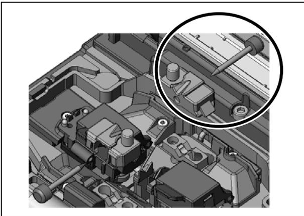
3: Lift the electrode cover plate as shown in the left figure.
