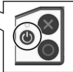
If you press the power key right after connecting the power cord to the power supply module, it may take a few seconds until the splicer is powered on.
