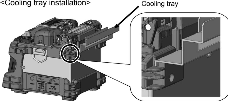
Install the cooling tray into the splicer as shown above.
