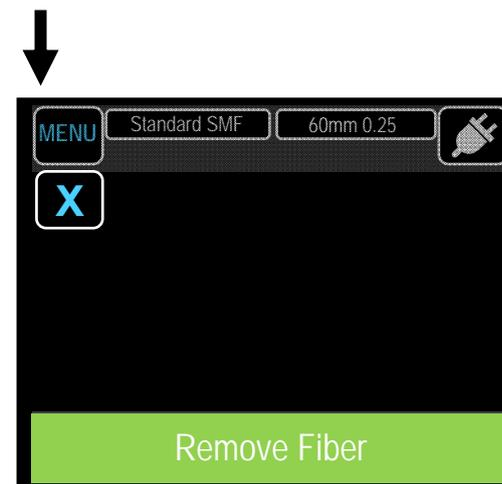
Open the hood and remove the spliced fiber when the screen above is displayed.
