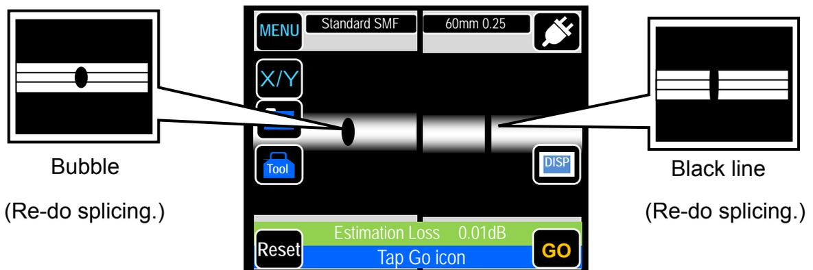
After MMF or dissimilar fiber splicing, a line sometimes appears at the splice point. But it does not affect splice quality, such as splice loss, tensile strength, and etc.
