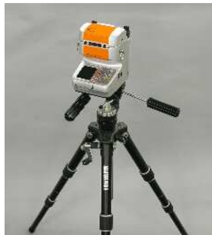
Attach a tripod to the splicer
