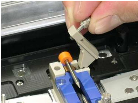
3. Remove the electrode cover plate.
