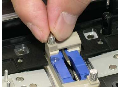
2. Using your fingers, loosen the thumbscrew.
