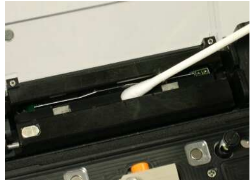
Clean the heat shrink oven with a dry cotton swab.
