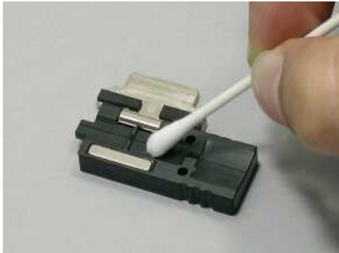
Clean the fiber holder with a cotton swab moistened with alcohol.
