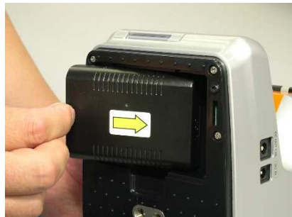
2. Install the battery as shown in the photo.
