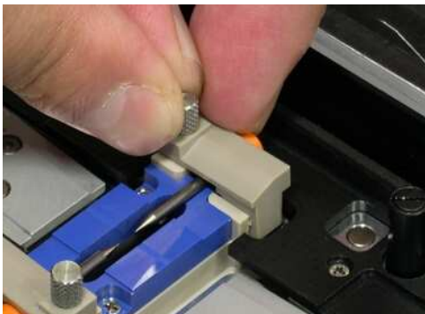
5. Install a new electrode. Tighten the thumbscrew while pushing the plastic button against the electrode cover plate.
