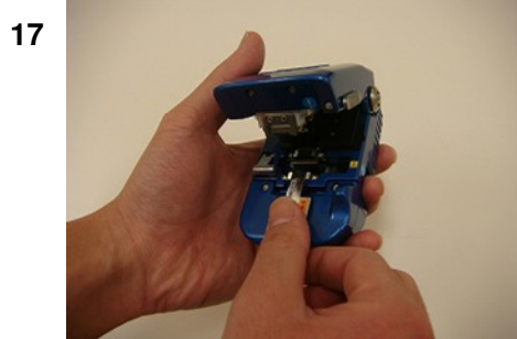
Set the fiber holder into the fiber cleaver.
