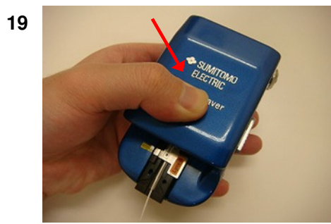
Close the cover of the fiber cleaver, cutting the glass fiber.
