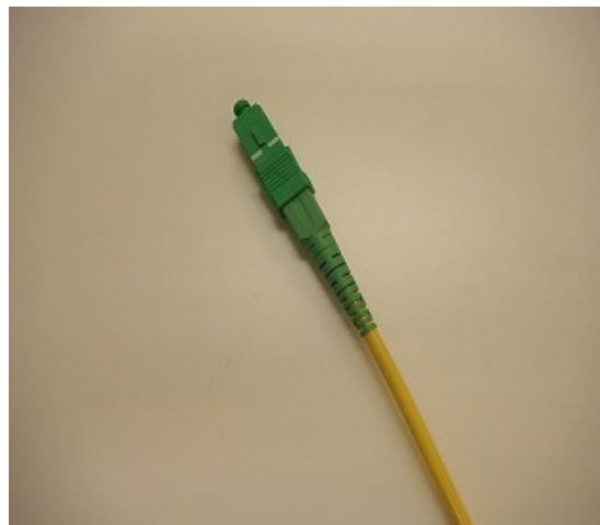
Put the outer housing over the inner housing. Align the notch of the outer housing with the notch of inner housing.
