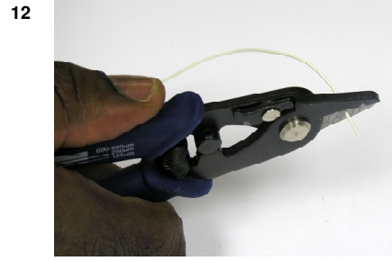
Strip the fiber coating to the marked point.
