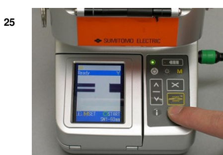
25 Ensure that the unit is set for single fiber splicing and 60mm sleeve setting.
