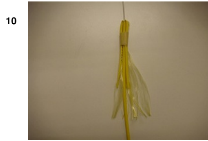
Fold the Kevlar and sheathing back.
