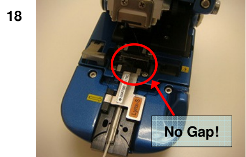
*Slide the front tip of the holder until it touches cleaver .
