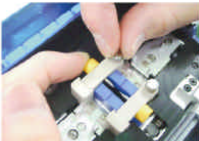
5. Tighten the screw while pressing the electrode collar on the V-groove.
