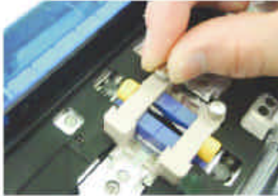
2. Loosen the electrode retainer screws, DO NOT try to remove the retainers from the base.
