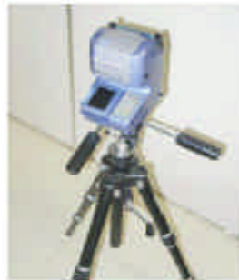
Ex. attach a tripod to the splicer
