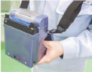
Ex. 1: Attach the strap to the upper 2 hooks.
