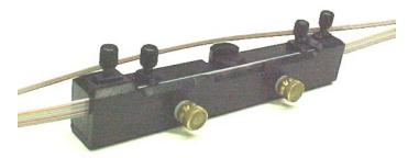
**5.2.6** Slide the round knob located in the center of the tool towards the ribbon, finishing at the 'closed' position beyond the ribbon slot. This sliding action splits the remaining 24-fiber ribbon into two 12-fiber ribbons.
