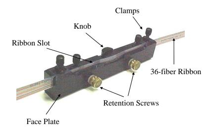
**5.2.3** Slide the round knob located in the center of the tool towards the ribbon, finishing at the 'closed' position beyond the ribbon slot. This sliding action splits the 36-fiber ribbon into two ribbons.
