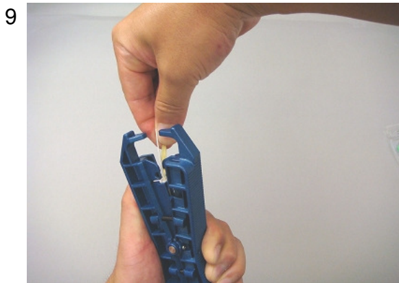
Pull the Kevlar and fiber to remove excess slack from inside cordage. Pull Kevlar to the side.
