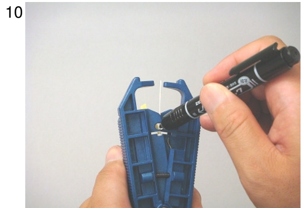
Using the hole of the tool as a gauge, mark the fiber . This mark represents the ending strip point and reference point for the holder edge.
